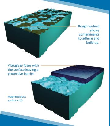
Vitroglaze acts as a barrier for your glass and 'smooths' its surface, inhibiting the growth of these contaminants and protecting your glass against harsh cleaners that can corrode and pit.
